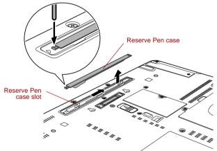
Figure 4-6 Removing the Reserve Pen case
